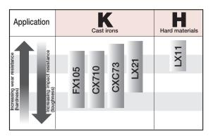
Our ceramics consist of high-purity fine powder oxides, nitrides, and carbides sintered through normal pressure, gas pressure and HIP sintering. The fine and dense structure ensures superiority in wear resistance, adhesion resistance, oxidation resistance and heat resistance.
